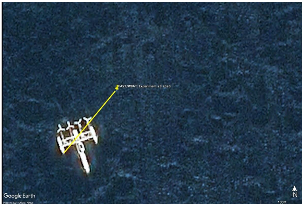
Figure 3.3.2: Deployment location of the WBAT echosounder mounted on the FAST platform, shown for Study 2B relative to the PLAT-I on a flooding tide. Length of yellow line represents the horizontal length from the optical camera and imaging sonar deployed at the leading edge of the starboard pontoon to the position of the FAST platform: \sim 60 m.
